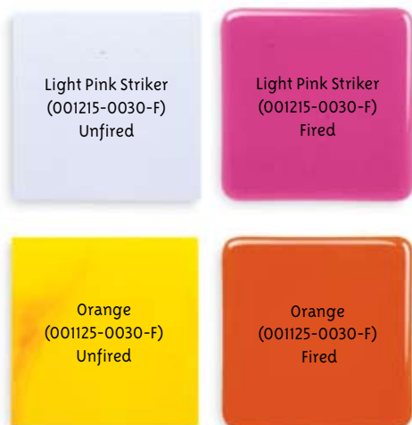
Some (but not all) of Bullseye's glasses appear pale but “strike” to the target color only after reheating. This example shows pieces of Light Pink Striker (001215-0030-F) and Orange (001125-0030-F) in the cold sheet (l), and after firing (r).
