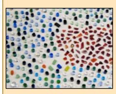
Little glass spheres can be made easily from either frit or rods. Nipped up rods create perfect spheres that have a tendency to be optically perfect. Protect a kiln shelf with a coat of kiln wash or piece of ThinFire<sup>TM</sup>. To make frit balls, scatter medium and coarse mesh frit on the kiln shelf making sure none of the pieces touch one another. To use
