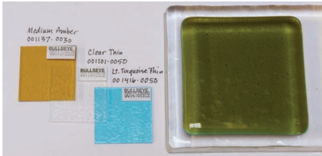
TOP: Medium Amber 001137-0030; MIDDLE: Clear Thin 001101-0050; BASE: Light Turquoise Thin 001416-0050. Requires Clear Thin between colors to prevent a dark color reaction. (Tile shown elevated on a clear billet for light transmission.)
