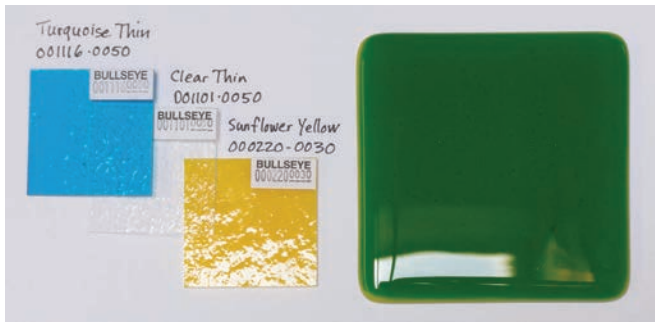
TOP: Turquoise Blue Thin 001116-0050 ; MIDDLE: Clear Thin 001101-0050; BASE: Sunflower Yellow Opal 000220-0030. Requires Clear Thin between colors to prevent a dark color reaction.
