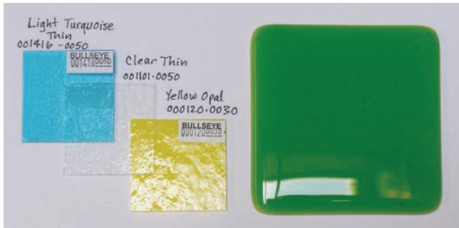
TOP: Light Turquoise Blue Thin 001416-0050; MIDDLE: Clear Thin 001101-0050; BASE: Yellow Opal 000120-0030. Requires Clear Thin between colors to prevent a dark color reaction.
