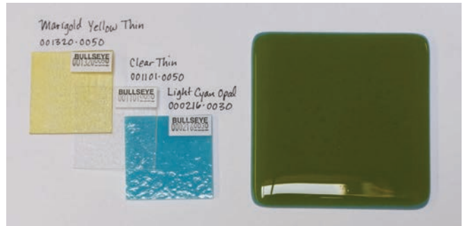
TOP: Marigold Yellow Thin 001320-0050; MIDDLE: Clear Thin 001101-0050; BASE: Light Cyan Opal 000216-0030. Requires Clear Thin between colors to prevent a dark color reaction.
