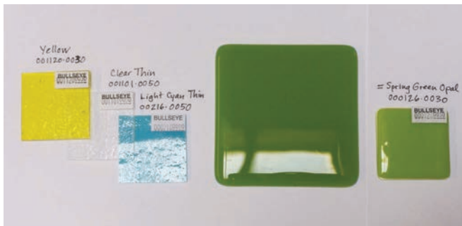
TOP: Yellow 001120-0030; MIDDLE: Clear Thin 001101-0050; BASE: Light Cyan Thin 000216-0050. Requires Clear Thin between colors to prevent a dark color reaction.
