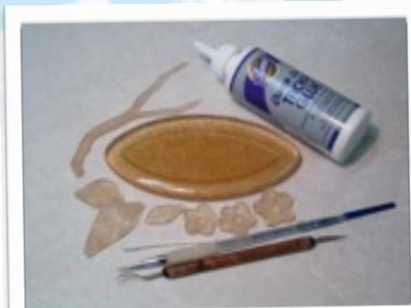
Since tack firing temperatures are hotter than slumping temperatures, there will be a tendency for the components to flatten. To prevent this from happening, cut small wedges of thick kiln paper. Slide the wedges under the folds in the components. Fire according to the Tacking Schedule. Note the slow ramp and the long annealing time. It is important to follow these slow ramps to avoid stressing and, perhaps, cracking the piece.
