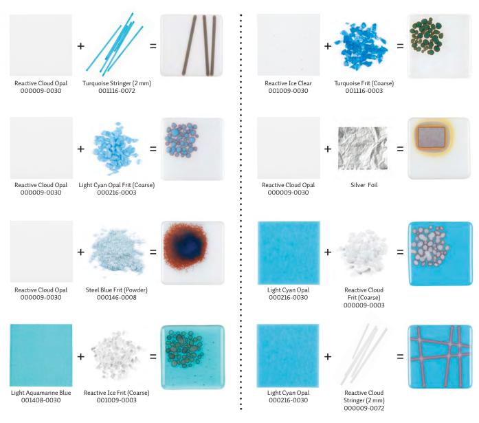
Layups: 6mm stacks (3 mm clear base + 3 mm reactive sheet), -0003 frit, 2 mm stringer, -0008 powder, Silver Foil Process temp: 1490°F (810°C)
