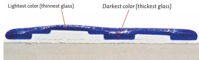
Figure 6: Cross-sectional view of kilnformed glass, fired at 1520°F (~825°C).
