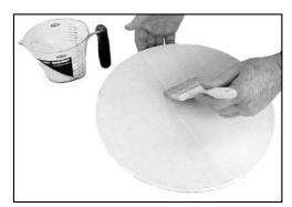
shelf. Four coats applied in opposite directions should be sufficient. Allow to dry for several minutes between coats. When you are finished allow them to dry completely before using. When they are completely dry they will have a uniform white appearance. **Never kiln wash the walls or lid of your kiln!**
