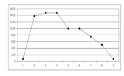
A firing program is composed of one or more firing segments that dictate the heating or cooling rate throughout the program.
