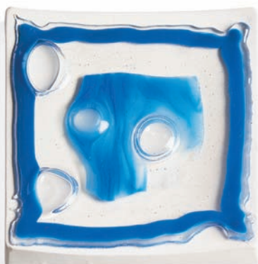
Figure 8 This plate was formed with a single firing for both fusing and slumping. This shortcut caused edge distortion and bubbles.
