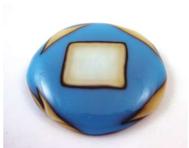
Given enough time and heat, the reaction between two glasses will spread, as in the square on the top of this piece. (Photo by the author.)
