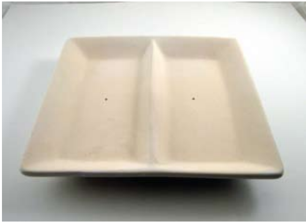
Molds with steep rims, such as this one, are difficult to use because the sides will draw in as the glass slumps. (Photo by the author.)
