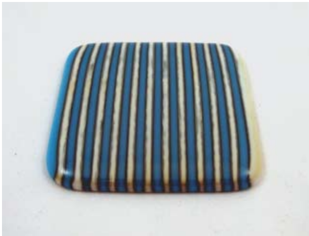
A typical reaction between a blue glass containing copper and a second french vanilla glass containing sulfur. The reaction creates the dark line where the two glasses touch. (Photo by the author.)
