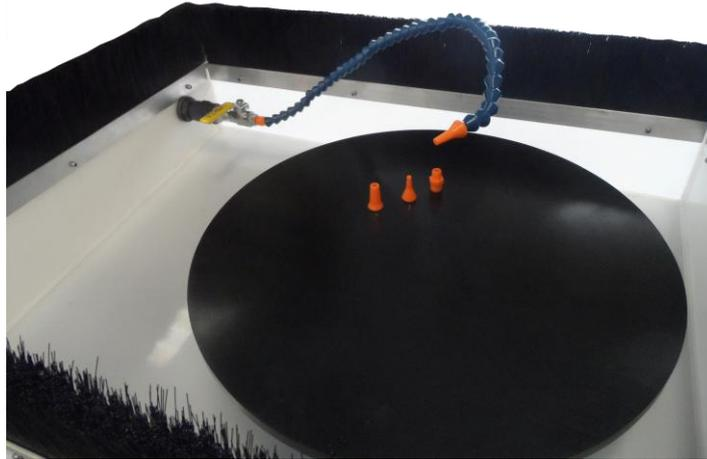
The MAG has a cast iron wheel head to accept adhesive backed or magnetic grinding disks. It is powered by an AC industrial motor through a V belt reduction drive and gearbox. Speed drive is controlled from a sophisticated AC inverter drive which gives an extremely smooth speed variation and high torque characteristics accompanied by extremely quiet operation.
