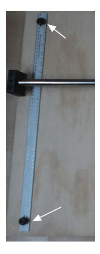
Put washer (E) on Thumbscrew (B) screw through ruler slots. Leave thumbscrews loose.
