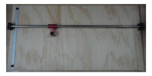
The mounting kit allows you to mount the Studio glass cutter on a plywood base so it can be moved when you are not using it.
