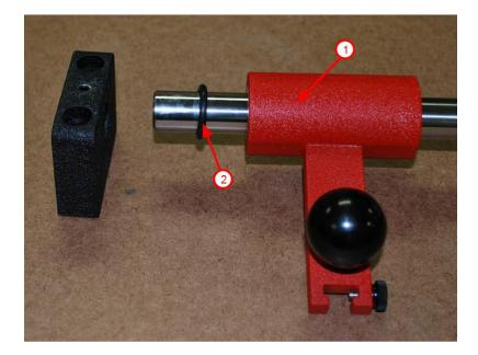
Before assembling clean the slide rod with WD 40 or a degreaser. Wipe down with a paper towel, and apply a thin coat of light oil.
