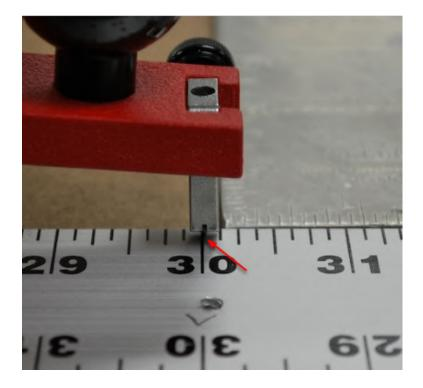
Line up your center mark on the ruler with the cutting wheel. Once it is centered, use the spring clamps to hold down the ruler.
