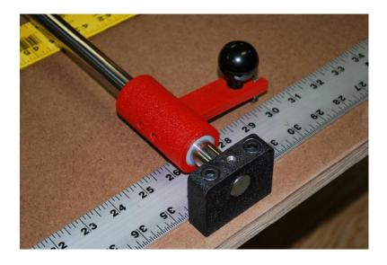
Install remaining bolts. Ttighten all 4 bolts, and the 2 set screws that hold the bar. The mounting of the cutter is complete.
