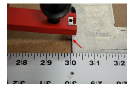
Slide the cutter about 1" away from the ruler. Make sure the framing square is pressed up against the ruler, and slide it until it touches the cutting head.
