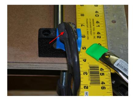
Use a c-clamp to hold the support to the table. It should be tight enough to hold the assembly from moving while drilling. repeat for other side.
