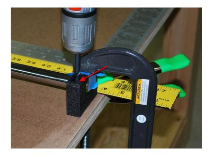
Use a 5/16" drill bit to drill through through the table. Drill slowly as not to mar the part when you drill through. If you are uncomfortable drilling all of the way through, drill 1/2 way through on both ends before removing cutter to complete holes.
