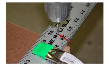
Start by drilling some mounting holes. I recommend drilling holes every 6" and 1/2" from each end. Use sand paper to remove the sharp edges after drilling.
