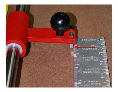
Adjust the ruler so that the cutting head is touching the framing square along the length, and the square is pressed up to the ruler. You are trying to have the ruler 90 degrees to the cutting head. Take your time
