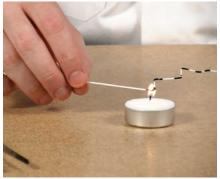
Always be cautious when using this process. The tip of the candle flame burns at around 1700°F (927°C), which is hot enough to soften the glass for manipulation.
