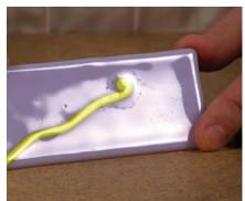
Wax is a contaminant that will show up in your finished work if not burned off prior to fusing.
