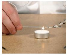
To get started, place the stringer in the tip of the flame. Hold it steady until the glass starts to soften.
