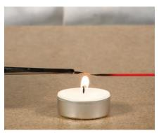
To create an elegant stringer terminus, hold the end in the flame with tweezers, keeping a very slight tension. When you feel the glass begin to soften, use the tweezers to pull while keeping the stringer in the flame.
