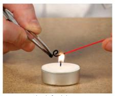
As you tap, slowly feed the stringer into the flame to heat up the next continuous section. Keep going until you have the desired size and shape.
